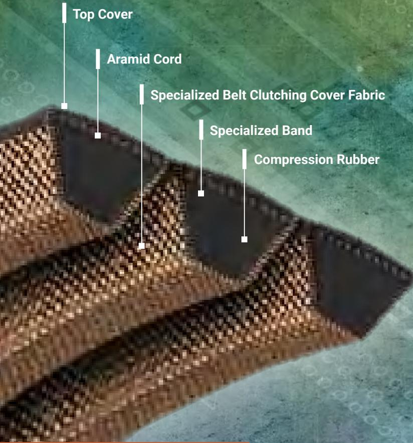
Mitsuboshi's **SUPER WEDGE II** V-belt is designed for heavy-duty applications where high torques need to be transmitted and shock loads can occur easily. By using a special rubber compound mixture, together with an aramid cord and a special cover fabric, we succeeded in developing the strongest belt for applications like road grinders and wood chippers.
